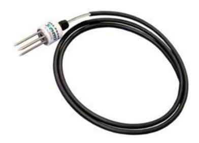
The SDI-SMT-2 Hydra probe offers a unique advantage over other soil probes by providing an all-in-one, in-situ system that can measure many different parameters simultaneously.
