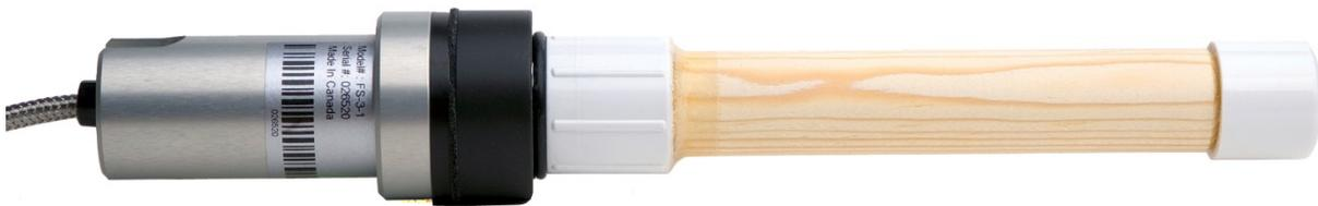
The FTS FS-3 electronic fuel stick sensor is commonly deployed on-site near prescribed burn and wildfire operations. The sensor’s output tracks closely with 10-hour fuel moisture, an invaluable indicator of fire behavior. The sensor uses digital compensation and linearization to provide a greater degree of precision and better temperature performance than analog sensors.
