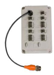
The FTS SDI-AM Analog Module is a flexible expansion interface that is compatible with a wide variety of analog sensors and any SDI-12 compliant datalogger/DCP such as the Axiom. It allows the Axiom to connect to virtually any analog sensor, and control power to a wide range of devices (ex. pumps, cameras, actuators, etc.).
