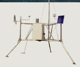
The fixed Remote Automated Weather Station (RAWS) is the standard for remote automated weather stations used in North America for fire weather monitoring. It is designed specifically with the interests of fire and fuels management agencies for use in remote areas, requiring only annual service and maintenance. From the assembly of a new station at a remote location to yearly service and maintenance, the design of the fixed RAWS shows our extensive 40 years of experience in the market.
