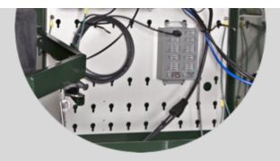
Back wall-mounted aluminum key-way plate facilitates quick yet secure mounting of system components like dataloggers.
