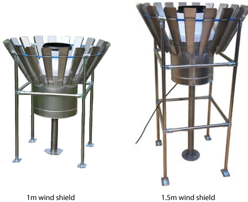
Figure 1-3: AWP with Wind Shield
