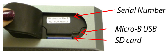
Figure 1-2: SD card and Micro-B USB port access
