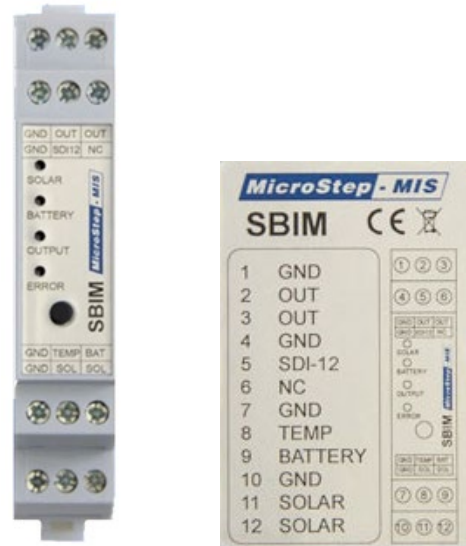
Figure 2-6: Solar regulator pin diagram
