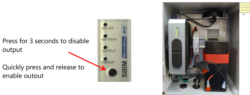
Figure 2-7: Solar Regulator status LEDs and final power connections (LT1-CELL2 shown)
